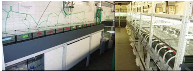
Fig. 2: Design of a semistatistic system and a flow through system.
